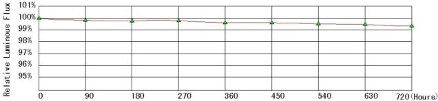
Based on the data obtained from an accelerated aging test over 720 hours with extreme temperature fluctuations, an average operating time of approx. 50,000 hours can be expected. The loss of light is less than 1% per 1000 hours
